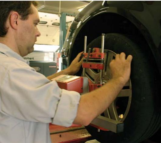
Tires are your car's critical connection to the road and can affect your ride, handling, traction and safety. Maintaining tire balance and wheel alignment reduces tire wear and improves handling and fuel economy.
