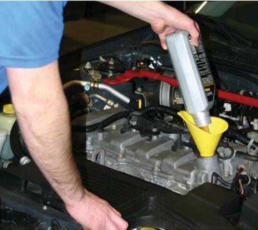
Critical parts of your engine are lubricated, cleaned and cooled by your car's oil and filter. Other specifically formulated fluids are used for the operation and protection of systems and components such as brakes, cooling, power steering, automatic and manual transmissions, and transfer cases. Your car may also be equipped with a variety of filters including those for the transmission, fuel system and interior ventilation.
